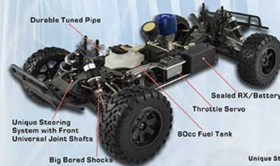
Single Speed (N1) Two Speed (N2) Diff Gearbox Set Front Universal Joint Shafts 3-piece design clutch shoes
